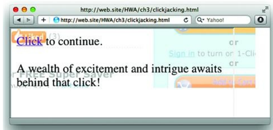
Figure 3.6 The overlay for a clickjacking attack
